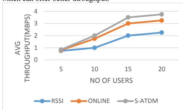
**Figure 3:** Resultant average throughput for RSSI, Online and S-ATDM techniques.
