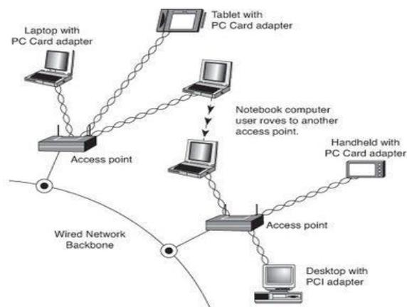
Fig 1: Infrastructure type WLAN
